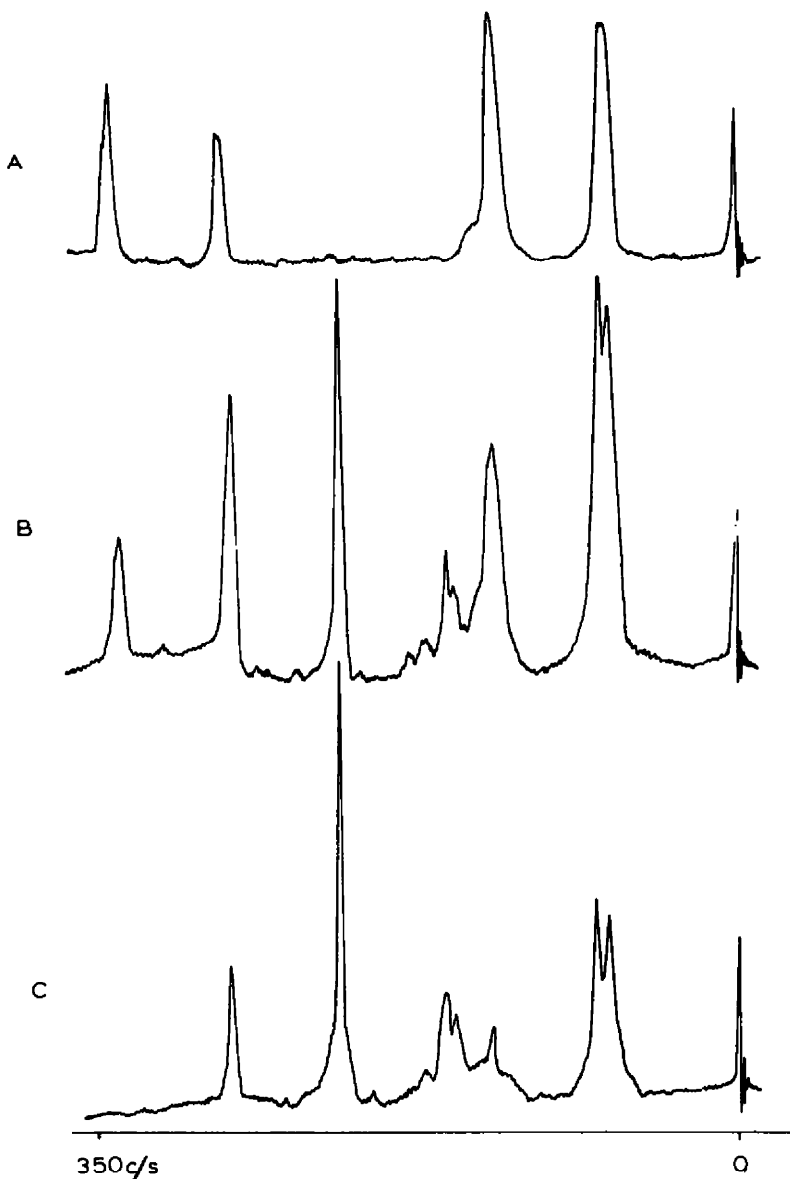
FIG. 1 Typical spectra obtained in C_6H_5N solution showing the region 0–340 c.p.s. from TMS. (A) Ergo flavin, (B) Ergochrysin B (equivalent to A + C), (C) Secalonic Acid B.
